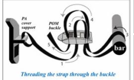
Step 3: Thread the strap through the buckle as shown. Repeat for the other strap.
